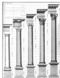
The Five Orders of Classical Architecture. From left, Tuscan, Doric, Ionic, Corinthian and Composite.
